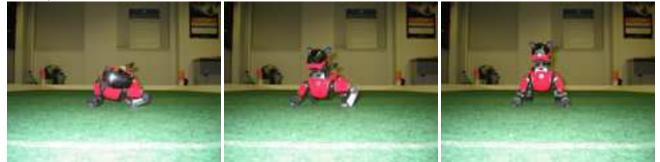
The head kick moves the ball almost due left (or right) a distance of up to 0.5 meters. We discovered that the head kick was especially useful when the ball was close to the edge of the field. The robot could walk to the ball, head kick the ball along the wall, and almost immediately continue walking, whereas the front power kick oftentimes kicked the ball against the wall, in essence moving the ball very little, if at all.
