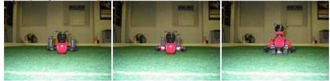
We found that the kick moves the ball relatively straight forward a distance of up to 3 meters. However, we noticed that the robot's front legs would miss the ball if the ball lies within 3 cm of the robot's chest. We resolved this issue by utilizing the robot's mouth to push the ball slightly forward before dropping its legs on the ball.
