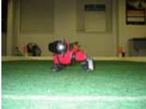
Finally, the robot leans in the direction of the kick as the head turns to kick the ball.
