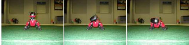
The robot then moves its front leg (left leg when kicking left, right leg when kicking right) out of the way.
