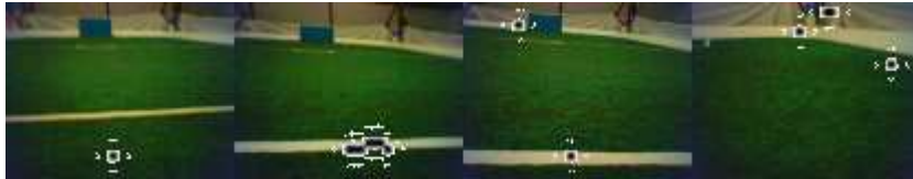
Fig. 5. Some typical errors on a field with no motion. In the run from which these images were taken, in which there was no motion on the field, 83% of the frames were correctly labeled as containing no motion.
