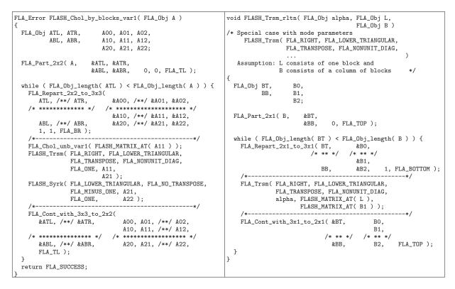
Figure 2: FLASH implementation of the Cholesky factorization and the corresponding triangular system solve.
