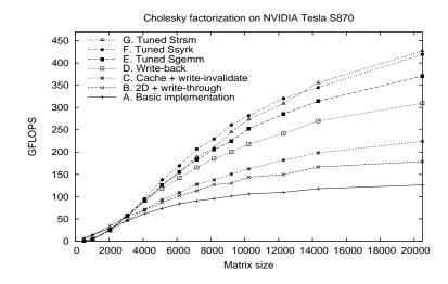
Figure 4: Performance of the blocked algorithm for the Cholesky factorization in the NVIDIA Tesla S870.
