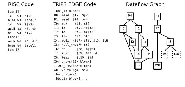
Figure 1: RISC and TRIPS code with dataflow graph.
