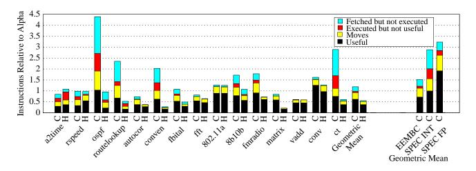
Figure 5: TRIPS instructions normalized to Alpha for compiled (C) and hand-optimized (H) benchmarks.
