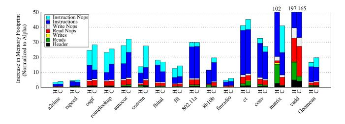
Figure 9: Increase in dynamic memory footprint for compiled (C) and hand-optimized (H) benchmarks.
