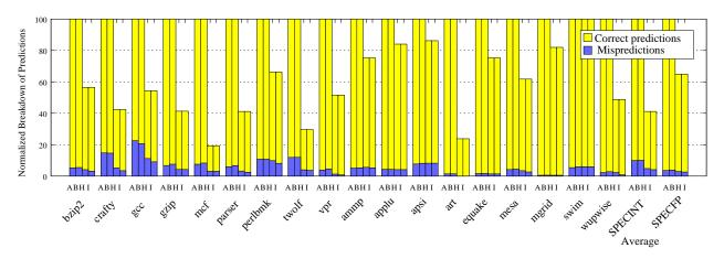
Figure 12: Block-predictor mispredictions normalized to total predictions made for basic blocks.
