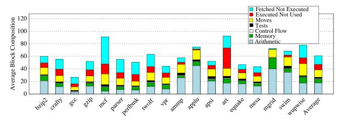
Figure 4: TRIPS block size and composition for compiled SPEC benchmarks.
