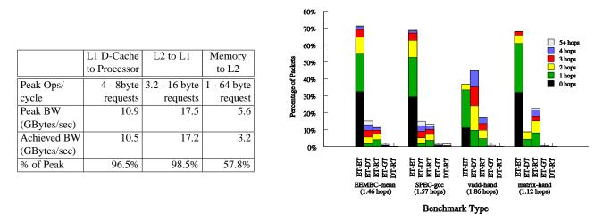
Figure 13: TRIPS bandwidths at 366MHz and operand network (OPN) profile with average hops per packet
