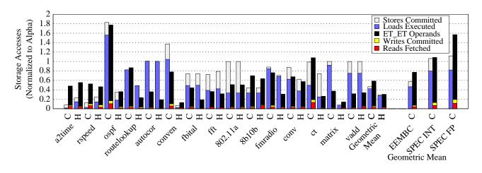
Figure 7: Storage accesses normalized to Alpha for compiled (C) and hand-optimized (H) benchmarks.
