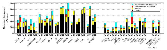
Figure 11: Average number of in-flight instructions for compiled (C) and hand-optimized (H) benchmarks.
