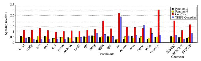
Figure 17: Speedup of TRIPS relative to the Core 2 on SPEC benchmarks.
