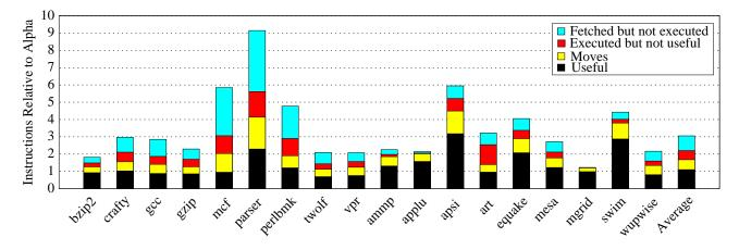
Figure 6: TRIPS instructions normalized to Alpha for compiled SPEC benchmarks.
