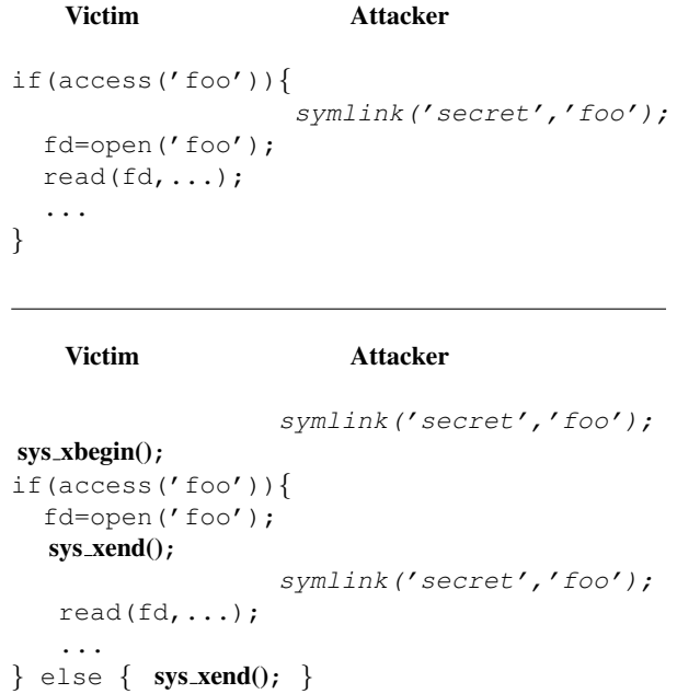
Figure 1: An example of a TOCTTOU attack, followed by an example of eliminating the race with system transactions. The attacker’s symlink is serialized (ordered) either before or after the transaction.
