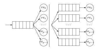
Figure 3: Depictions of a single-queue multi-server system (left) and a multi-queue multi-server system (right) each with p processing elements.
