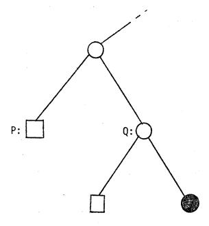
Figure 1. The block at the address of the buddy of the block at P is available, but the buddy of the block at P (at Q) is not available. Squares (耳) indicate available blocks; Circles indicate blocks reserved by the user (•), or blocks split into buddies (o).
