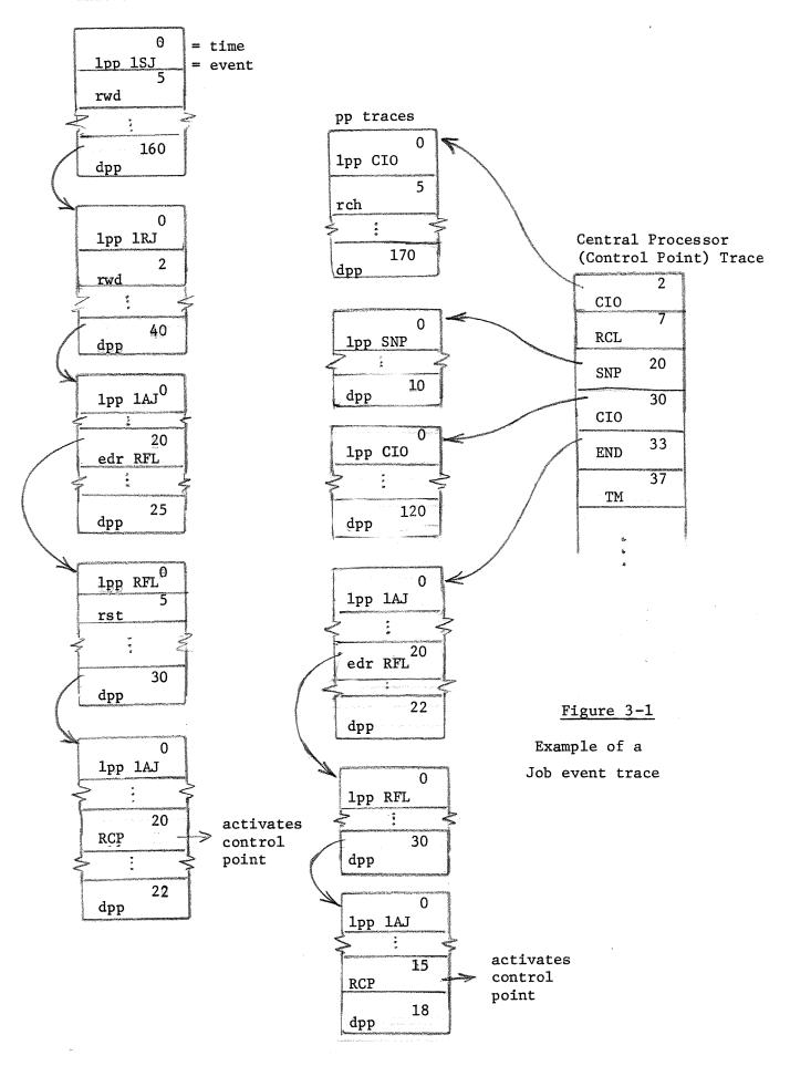
for the job before the CP was ever activated. The 'Recall Central Processor' event in a PP sequence (invocation type 8) represents the enabling of the central processor. It does not include a link to the central processor in the job trace, because due to lack of synchronization of the PP and CP, this PP event cannot specify the particular point at which CP processing should resume.
