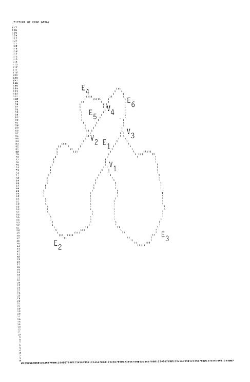
Figure 1. An edge picture containing two objects, four vertices, six edges, and four surface boundaries.
