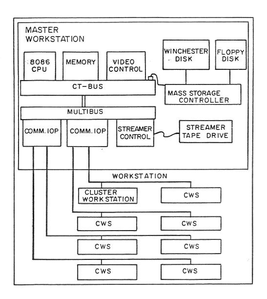
Figure A9. Convergent technologies multifunction workstation.
