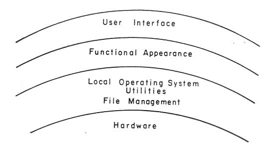
Figure 2. The various levels of organization in a workstation.
