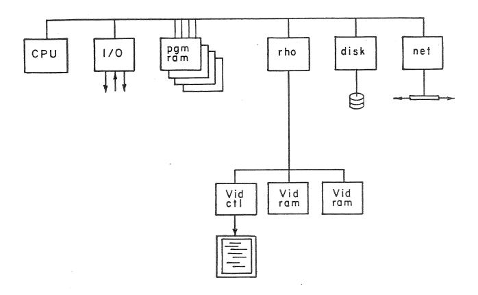
Figure A2. A system configuration based on the Nu bus.
