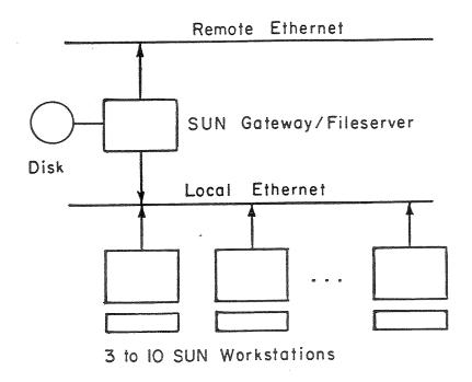
Figure A4. A configuration of SUN workstations.
