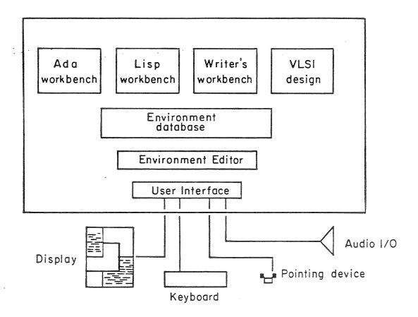
Figure A8. The levels of software organization in a SPICE workstation environment.
