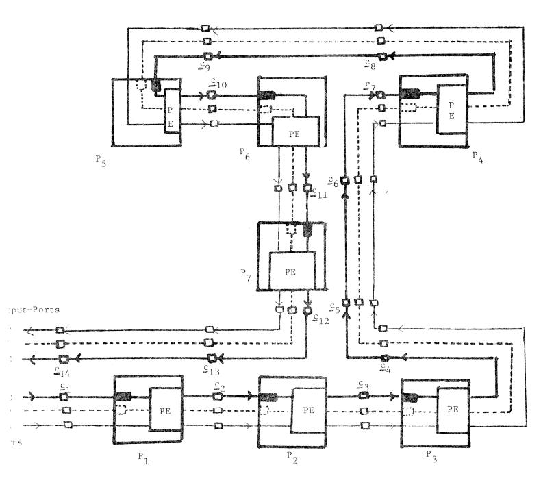
Figure 2(b): Configuration of shift registers and processing elements corresponding to Figure 1(b)
