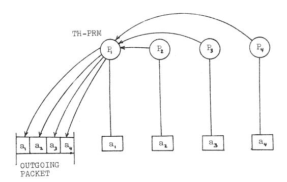
Figure 4-3: Packet Assembly
