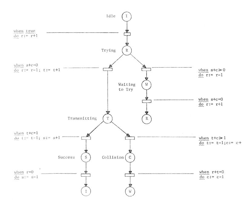
Figure 3 A labeled Petrinet that models the nonpersistent CSMA protocol
