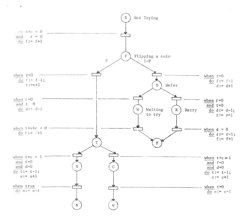
Figure 5 A labeled Petrinet that models the P-persistent CSMA protocol. (For one-persistent CSMA, the enabling predicate of  $t_{\rm FD}$  is modified from r=0 to false.)
