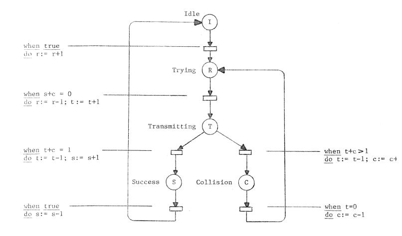
Figure 4 A labeled Fetrinet that models the virtual time CSMA protocol
