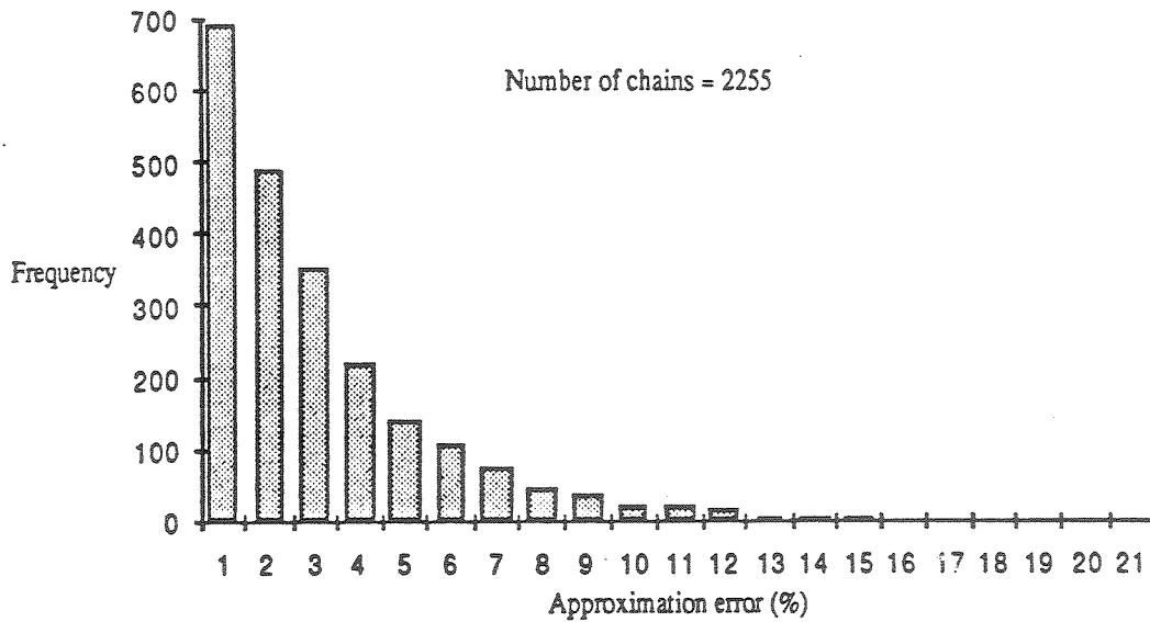
Figure 9. Distribution of approximation errors of throughputs of individual chains calculated by PAM_IMPROVED for the 100 networks.
