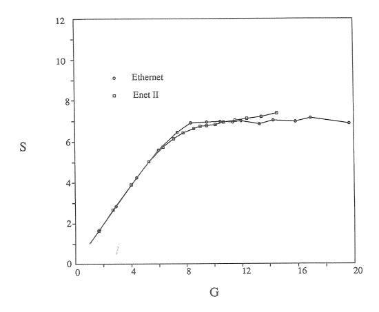
Figure 6. Throughput (S) versus offered channel load (G) for five generators sending mixed length packets. X and Y axis units = megabits per second.
