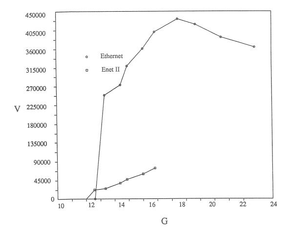
Figure 5b. Delay variance (V) versus offered channel load (G) for four generators sending 1500 byte packets. Y units = microseconds, X units = megabits per second. Heavy overload conditions.
