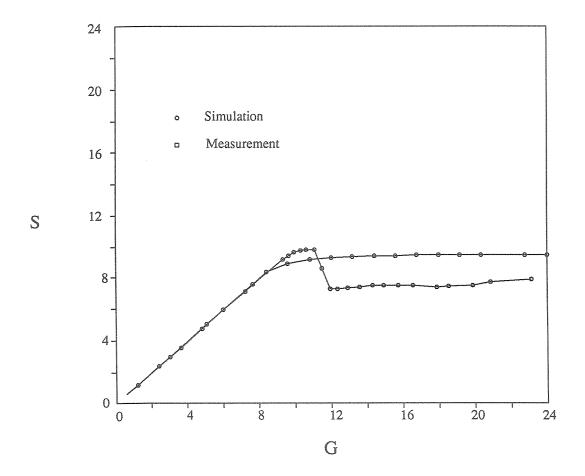
Figure 9. Throughput (S) versus offered load (G) for simulated and measured Ethernet. 1500 byte packets, x and y axes in Mbps.
