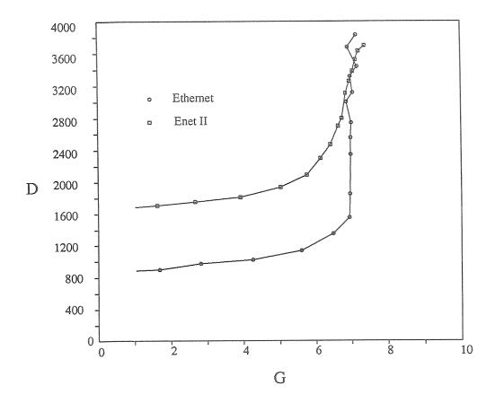
Figure 7. Queueing delay (D) versus Throughput (S) for four generators sending mixed length packets. X axis units = megabits per second. Y axis units = microseconds
