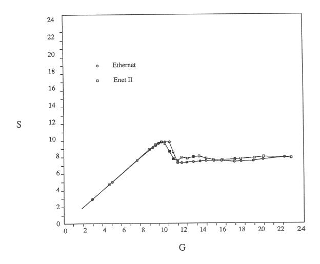
Figure 3. Throughput (S) vs. offered channel load (G) for five generators sending 1500 byte packets. X and Y axis units = megabits per seconds.
