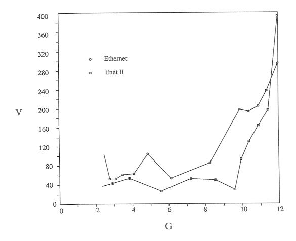
Figure 5a. Delay variance (V) versus offered channel load (G) for four generators sending 1500 byte packets. Y units = microseconds, X units = megabits per second. Normal operating range.
