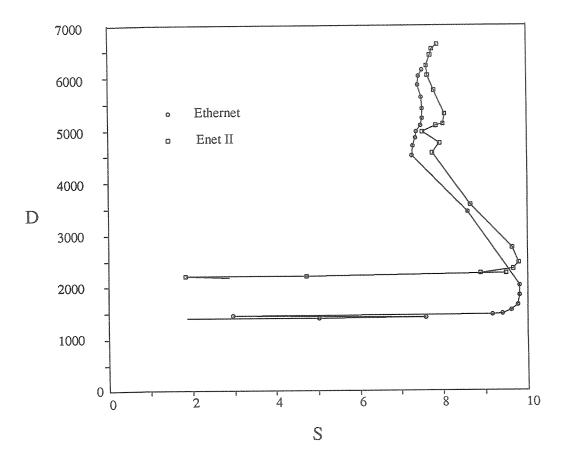
Figure 4. Packet queueing delay (D) versus Throughput (S) for five generators sending 1500 byte packets. X units = megabits per second, Y units = microseconds.
