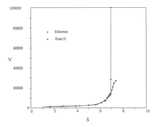
Figure 8. Queueing delay variance (V) versus Throughput (S) for five generators sending mixed length packets. X axis units = megabits per second. Y axis units = microseconds
