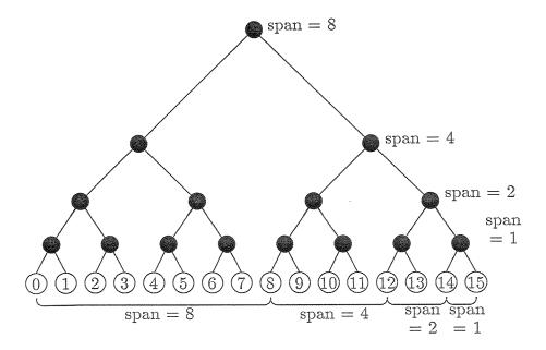
Figure 1: Original KYKLOS-II topology illustrating span:  $N=16,\,r=1.$
