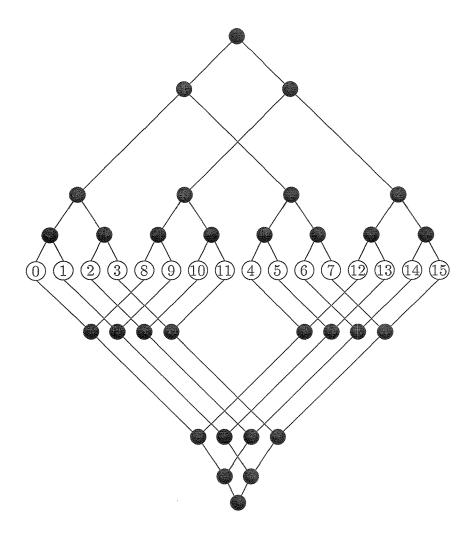
Figure 5: Proposed KYKLOS-II network of Figure 3, relabeled in accordance with Figure 4. If it is twisted to remove the cross-over from the upper tree, this network becomes equivalent to the original KYKLOS-II network shown in Figure 2.
