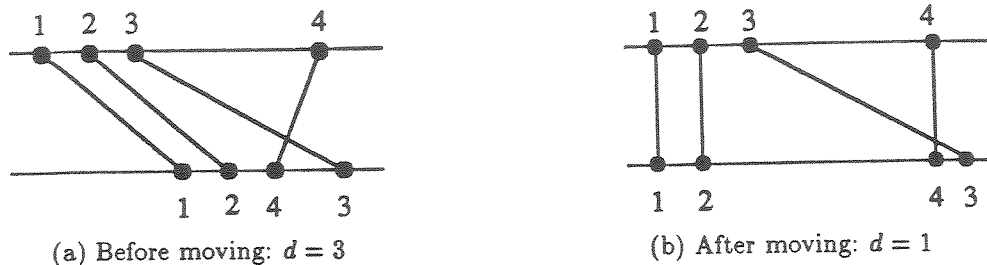
Figure 1: Reducing channel density by moving terminals
