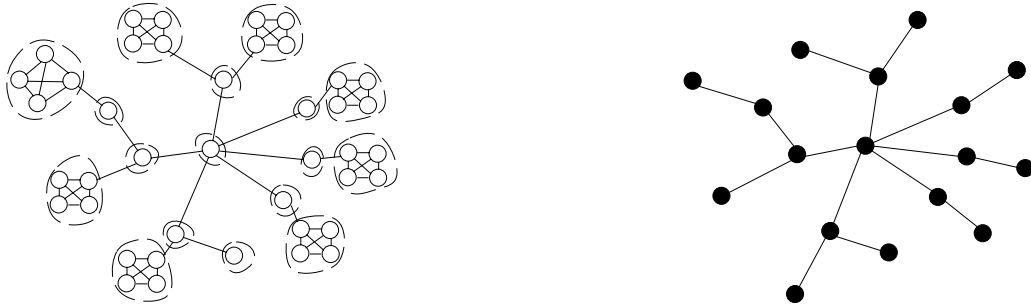
Figure 7.1: Illustrating a 2-edge-connected graph (on the left) and its 2\text{-}ebk(G) (on the right). Note that the 2\text{-}ebk(G) is a tree-like structure and vertex 10 is shared by three cycles.
