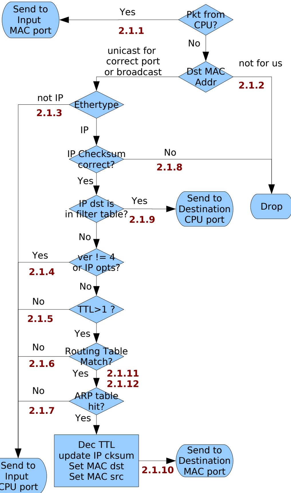
**Software Component Of NETFPGA Reference Router**
