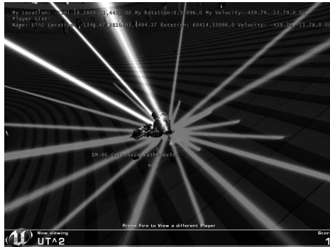
Fig. 3 Ray-Tracing Level Geometry Sensors. Gamebots has a debugging option for viewing ray traces on a bot. The figure shows all 22 ray trace sensors around the bot, with the contrast heightened to improve visibility. Some of the rays aiming upward are brighter because they are not colliding with any level geometry. These sensors provide the bot with information about the structure of its immediate environment, which helps it reason about how best to dodge enemy attacks. Though disabled in BotPrize 2010, these sensors should help the bot be more aware of its surroundings in future competitions.
