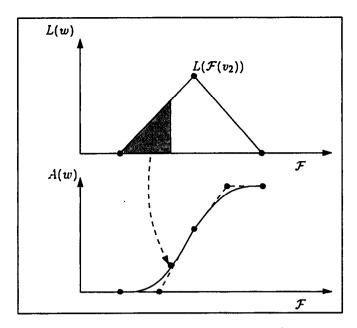
Figure 3: 2D area computation by integration of the length function L(w). The shaded region corresponds to the area *less than* or *below* the isovalue. The area *above* the isovalue is computed symmetrically.
