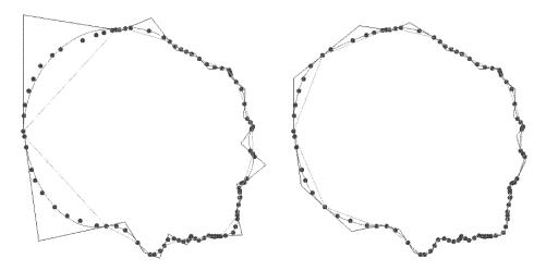
Fig. 4.  $G^3$  cubic A-splines fit of head data with different approximation errors. The picture on the left has fewer number of pieces and has larger error than the picture on the right.
