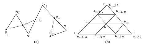
Fig. 1. (a) A  $G^1$  polygon; (b) Bézier coefficients of cubic.
