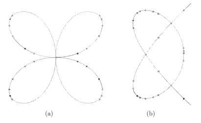
Fig. 6. A-spline approximation of implicit algebraic curves: (a)  $(x^2 + y^2)^3 - 4x^2y^2 = 0$ ; (b)  $x^3 - 3x - (1/9)(y^4 - 12y^2 + 18)$ . The curve segments between consecutive vertices (dots) are all cubic degree and with  $G^3$  continuity at the vertices.
