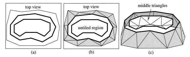
Fig. 9. An untiled region occurs at an appearing/disappearing vertical feature. Shaded regions show the tiling triangles. (a) The thick contours are on the top slice. (b) The inner top contour is untiled. (c) Perspective view of the constructed surface. The untiled region is covered by middle triangles.
