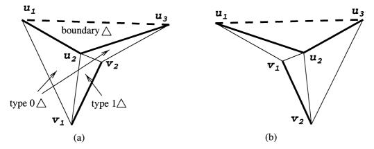
Fig. 17. Untetrahedralizable shapes defined in Lemma 5: (a) reflex  $\overline{u_2v_2}$ ; (b) reflex  $\overline{u_2v_1}$ .
