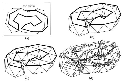
Fig. 24. This shows the tetrahedralization of a solid containing a dissimilar region (the inner portion of the top contour). The interior of the dissimilar region is void. (a) The thick contour is on the top slice. (b) The reconstructed surface mesh. (c) Tetrahedralization. (d) The tetrahedra are separated for better visualization.
