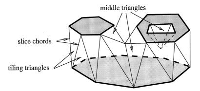
Fig. 6. The shaded regions are planar solid regions. The constructed surface consists of all non-planar triangles.
