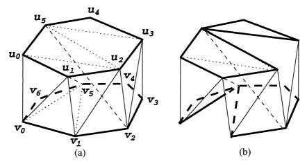
Fig. 13. Forming tetrahedra using non-boundary triangles often makes the remaining part untetrahedralizable. (a) Two tetrahedra formed using non-boundary triangles  $u_2u_3u_5$  and  $v_0v_1v_5$ . (b) The remaining part.
