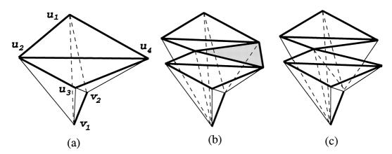
Fig. 19. Untetrahedralizable prismatoids which have two top boundary triangles and no bottom triangle: (a) the simplest case; (b) one variation which has non-boundary triangles between two top boundary triangles; (c) if a tetrahedron is formed using a non-boundary triangle (e.g. the shaded triangle in (b)), the remaining part becomes very irregular.
