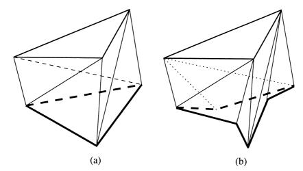
Fig. 2. (a) An untetrahedralizable Schönhardt prism; (b) AFT could result in a more irregular remaining part.
