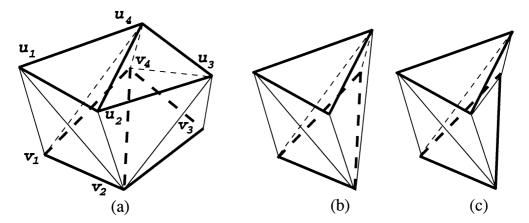
Fig. 18. (a) A prismatoid in which  $\overline{u_1v_2}$  and  $\overline{u_4v_1}$  are reflex.  $\Delta u_4u_1v_2$  is protected. (b) No tetrahedra can be formed via our operator to cut across  $\Delta u_4u_1v_2$ . (c) The protection rule prohibits the generation of this untetrahedralizable remaining part because  $\Delta u_4u_1v_2$  is cut across by  $\overline{u_2v_4}$ .
