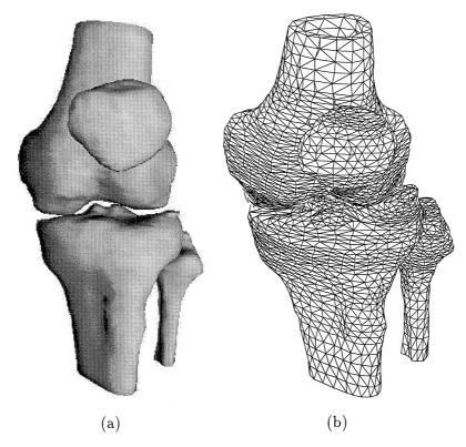
Fig. 31. A knee joint consisting of the lower femur, the upper tibia and fibula and the patella: (a) Gouraud shaded; (b) the tetrahedralization.
