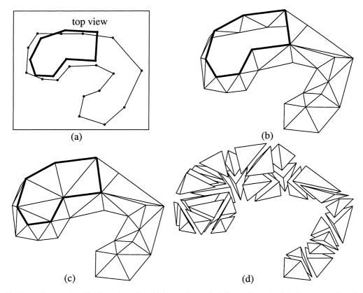
Fig. 23. This shows the tetrahedralization of a solid which contains a dissimilar region (the right bottom portion of the bottom contour). The interior of the dissimilar region is solid. (a) The thick contour is on the top slice. (b) The reconstructed surface mesh. (c) Tetrahedralization. (d) The tetrahedra are separated for better visualization.
