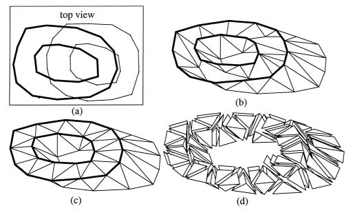
Fig. 28. This shows the processing of nested prismatoids. (a) The thick contours are on the top slice. (b) The reconstructed surface mesh. (c) Tetrahedralization. (d) The tetrahedra are separated for better visualization.
