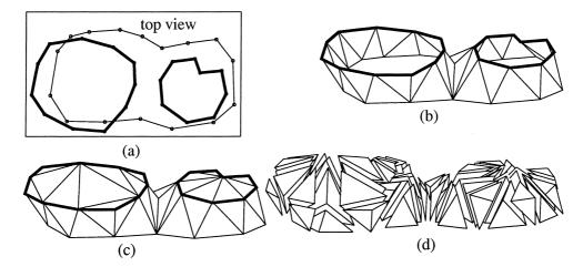
Fig. 21. This shows the tetrahedralization of a solid which contains a one-to-many branching. (a) The thick contours are on the top slice. (b) The reconstructed surface mesh. (c) Tetrahedralization. (d) The tetrahedra are separated for better visualization.
