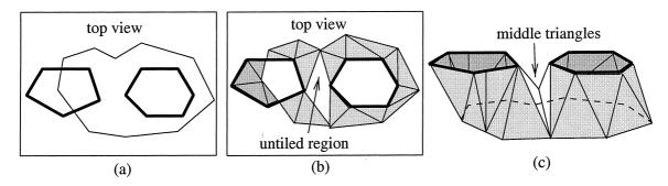
Fig. 7. An untiled region occurs at branching region. Shaded regions shoe the tiling triangles. (a) The thick contours are on the top slice. (b) The branching region is untiled. (c) Perspective view of the constructed surface. The untiled region is covered by middle triangles.
