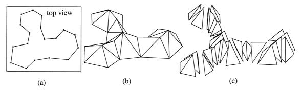
Fig. 25. This shows the tetrahedralization of a solid which contains an appearing/disappearing vertical feature of a solid interior. (a) The contour is on the bottom slice, and it has no corresponding contour on the top slice. (b) The reconstructed surface mesh. (c) The tetrahedra are separated for better visualization.
