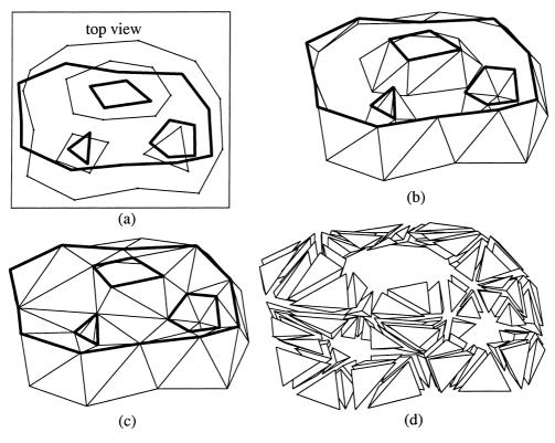
Fig. 29. This shows the processing of multiply nested prismatoid. (a) The thick contours are on the top slice. (b) The reconstructed surface mesh. (c) Tetrahedralization. (d) The tetrahedra are separated for better visualization.
