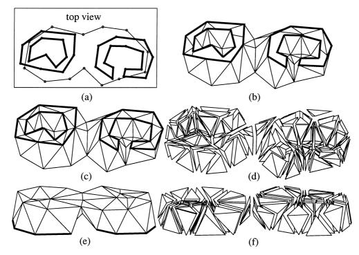
Fig. 27. This shows the tetrahedralization of a solid which contains a branching, a disimilar portion (the inner portion of the top right contour), and an appearing/disappearing vertical feature (the inner contour at the left of the top slice). (a) The thick contours are on the top slice. (b) The reconstructed surface mesh. (c) Tetrahedralization. (d) The tetrahedra are separated for better visualization. (e) and (f) are viewed from the bottom.
