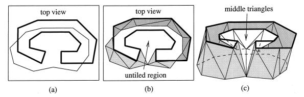
Fig. 8. An untiled region occurs at a dissimilar portion of a contour. Shaded regions show the tiling triangles. (a) The thick contour is on the top slice. (b) The dissimilar portion is untiled. (c) Perspective view of the constructed surface. The untiled region is covered by middle triangles.
