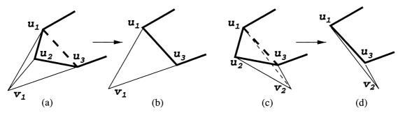
Fig. 15. The weight factor. (a) and (c) show forming a tetrahedron, and (b) and (d) show the their remaining part, respectively. The weight factor of (a) is smaller than 1 and that of (c) is larger than 1.
