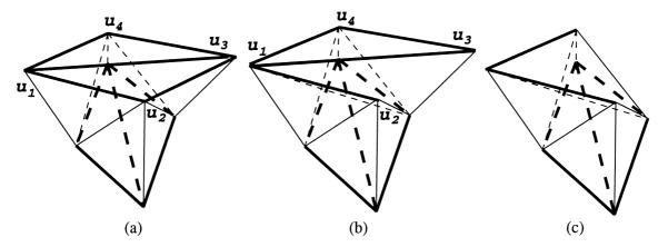
Fig. 16. Our group operator can avoid generating an irregular remaining part. (a) It is untetrahedralizable by our group operator. (b) The remaining part after forming one tetrahedron. (c) The remaining part after forming two tetrahedra.
