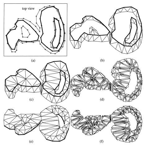
Fig. 30. This shows the tetrahedralization of the solid region between two slices of a human tibia. The distance between slices is enlarged 5 times. The reconstructed shape includes a branching and a appearing/disappearing vertical feature. (a) The thick contours are on the top slice. (b) The reconstructed surface mesh. (c) Tetrahedralization. (d) The tetrahedra are separated for better visualization; (e) and (f) are viewed from the bottom.
