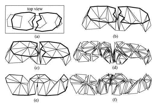
Fig. 22. This shows the tetrahedralization of a solid which contains a many-to-many branching. (a) The thick contours are on the top slice. (b) The reconstructed surface mesh. (c) Tetrahedralization. (d) The tetrahedra are separated for better visualization. (e) and (f) are viewed from the bottom.
