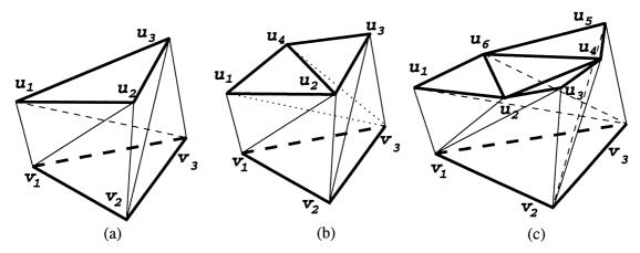
Fig. 20. The untetrahedralizable prismatoids have one bottom triangle. (a) the simplest form which is a Schönhardt prism; (b) and (c) are two variations. (b) To be untetrahedralizable, the prismatoid must be irregular enough so that both  $\overline{u_4v_2}$  and  $\overline{u_3v_1}$  are partly outside it. (c) None of  $\overline{u_2v_3}$ ,  $\overline{u_4v_1}$ ,  $\overline{u_6v_2}$ ,  $\overline{u_3v_3}$ ,  $\overline{u_1v_2}$ , and  $\overline{u_5v_1}$  is totally inside the prismatoid.
