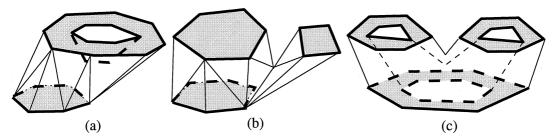
Fig. 11. Three examples which cannot be reduced into prismatoids by our algorithm because the projections of the middle vertices onto the bottom slice do not fall inside a planar solid region (the shaded region).
