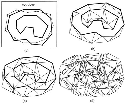
Fig. 26. This shows the tetrahedralization of a solid which contains an appearing/disappearing vertical feature (the top inner contour) of a void interior. (a) The thick contour is on the top slice. The top inner contour has no corresponding contour on the bottom slice. (b) The reconstructed surface mesh. (c) Tetrahedralization. (d) The tetrahedra are separated for better visualization.
