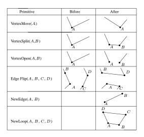
Figure 4: Isocontour refinement primitives.
