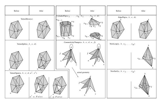
Figure 6: Isosurface refinement primitives.
