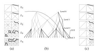
Figure 10: (a) Sequence of levels of resolution of an isocontour  $\mathcal{I}$  (bold black line) of a 2D scalar fieled (light gray liens). (b) The hierarchical representation of  $\mathcal{I}$  (black arrows) is a subgraph of the mesh hierarchy (gray arrows). (c) An adaptive refinement of  $\mathcal{I}$ .
