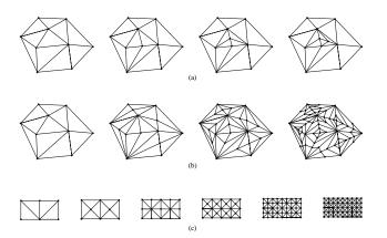
Figure 2: 2D Mesh refinement by edge-bisection. (a) Local adaptive refinement. (b) Global uniform refinement. (d) Sequence of edge-bisection refinements for a regular grid.
