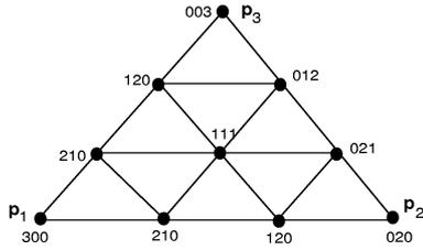
Fig. 4. Cubic coefficient index on the triangle  $[p_1 p_2 p_3]$ .
