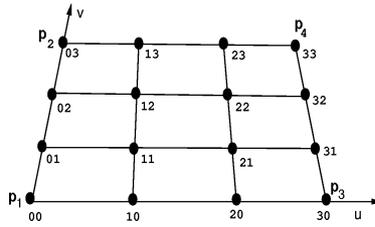
Fig. 5. Bi-cubic coefficient index on the quadrilateral  $[p_1 p_2 p_3 p_4]$ .
