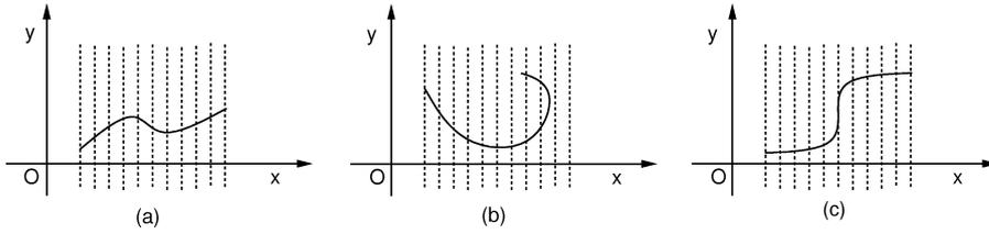
Fig. 10. (a) Single-valued regular function; (b) Multi-valued non-regular function; (c) Function not differentiable.
