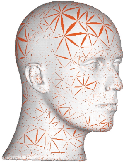
Fig. 14. Edge patches and face patches for a head.
