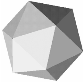
Fig. 12. Regular 20-faces polyhedron as a discretization of sphere.
