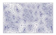
$\label{eq:Figure 9: The quadrilateral mesh after recursive quad subdivision refinement$
