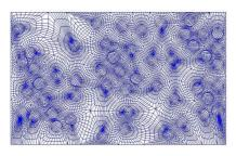
$\label{eq:Figure 10: The quadrilateral mesh after several steps of subdvision refinement$
