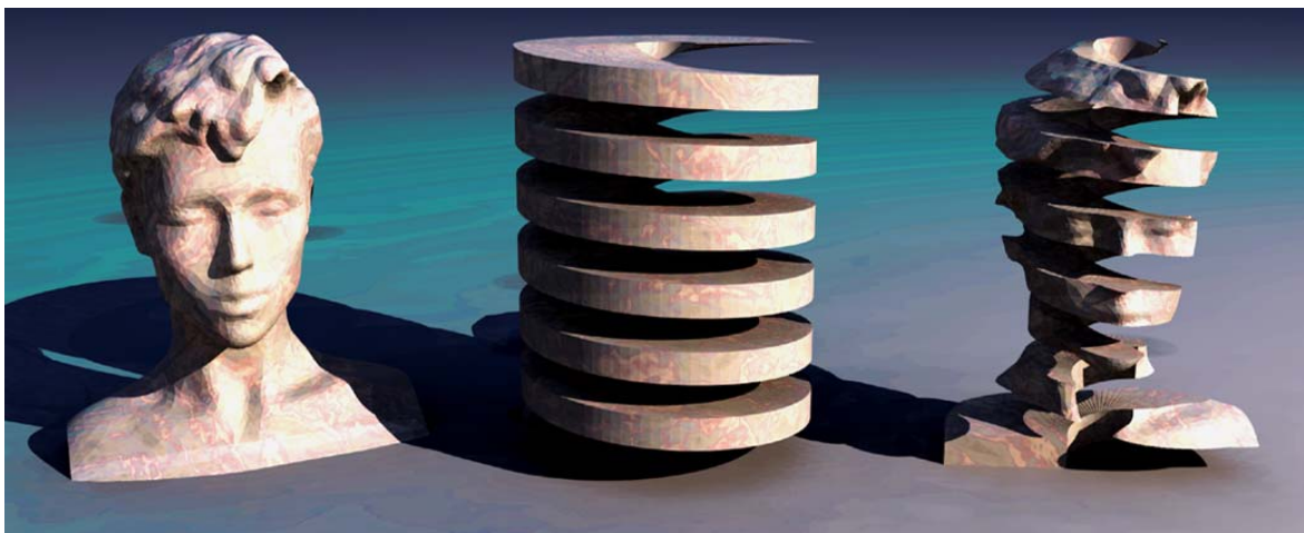
Fig. 1. (a) BSP tree generated from a polygon B-rep with normals; (b) solid helicoid; (c) progressive intersection.
