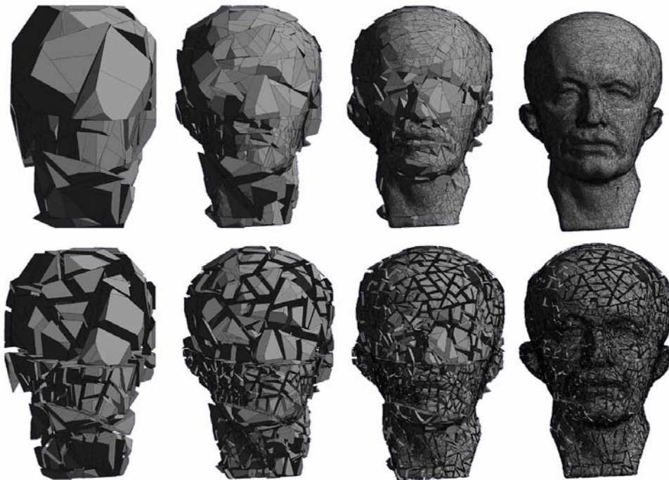
Fig. 9. Progressive transformation from B-rep triangles to BSP: (a) progressive solid models of the Max Plank head; (b) exploded views of the produced BSP.
