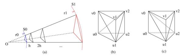
Fig. 12. (a) One triangle in the sphere  $S_0$  (blue) is extended n steps until arriving at the sphere  $S_1$  (red); (b), (c) a prism is decomposed into three tetrahedra in two different ways. (For interpretation of the references to color in this figure legend, the reader is referred to the web version of this article.)
