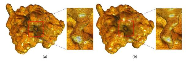
Fig. 14. Comparison of mAChE (9308 vertices, 18612 triangles) before and after surface mesh regularization. (a)—Original; (b)—after mesh regularization.
