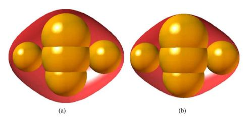
Fig. 6. The left picture shows the inflation effect by the Gaussian map. The right one shows the tight enclosure of atoms. The centers of the five atoms are (-2,0,0), (2,0,0), (0,-1,0), (0,1,0) and (0,0,0). The corresponding radii are 0.8,0.9,1.1,1.3 and 1.3. The parameter p in the Gaussian map is chosen to be 0.4. The tight approximation on the right figure is obtained by shrinking the five radii into 0.55644,0.72525,0.60476,1.04567 and 0.0 respectively. The unit is Angstrom.
