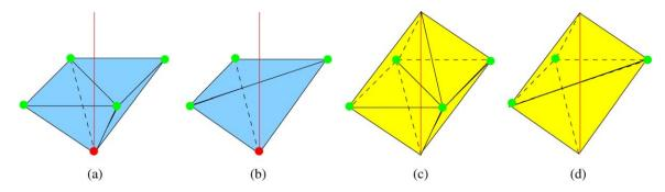
Fig. 11. Sign change edges and interior edges are analyzed in 3D tetrahedralization. (a), (b) Sign change edge (the red edge); (c), (d) interior edge (the red edge). The green solid points represent minimizer points, and the red solid points represent the interior vertex of the sign change edge. (For interpretation of the references to color in this figure legend, the reader is referred to the web version of this article.)
