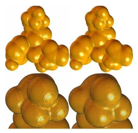
Fig. 13. The surface comparison before/after quality improvement. The left column shows the original surface of an ASN-THR-TYR peptide, and the right column shows the surface after mesh regularization. The top row shows the smooth shading surfaces, and the bottom row shows snapshots of the meshes.
