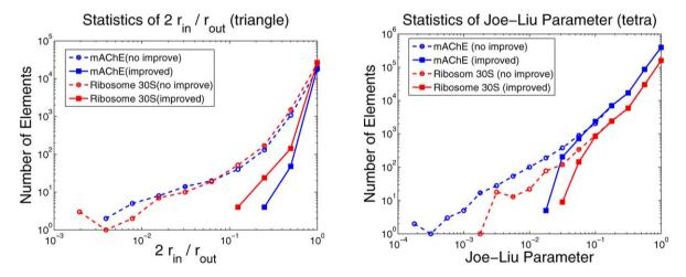
Fig. 16. The histogram of the aspect-ratio and Joe-Liu parameter.
