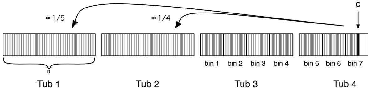
Figure 5: Illustration of the tub protocol from peer  $c$ 's perspective. Shaded entries represent peers that  $c$  can contact for a trade when appropriate. Note that  $c$  only uses bins for its own tub and the immediately preceding one.
