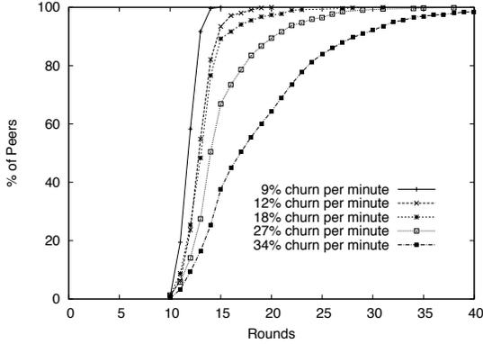
Figure 13: Join delay under churn. ( $n = 443$ )
