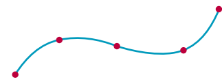
FIGURE 3-32 A spline curve formed with individual cubic polynomial sections between specified coordinate positions.
