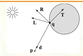
A ray is defined by an origin P and a unit direction d and is parameterized by t:
