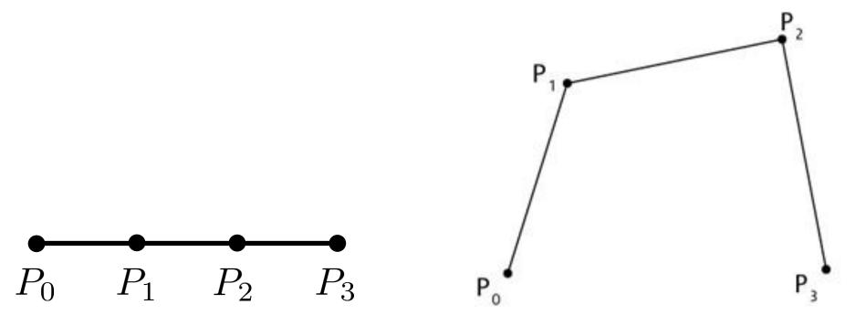
Main idea: recursive linear interpolation Start with four points – **control polygon** Clip corners
