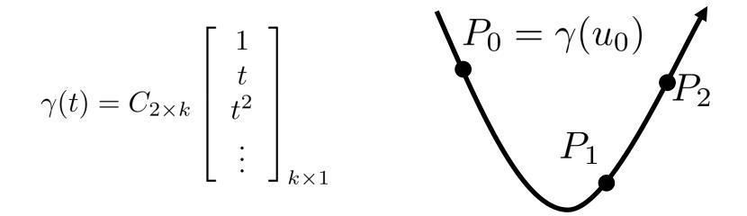
Notice: each coordinate is **linear combination** of a power of t
