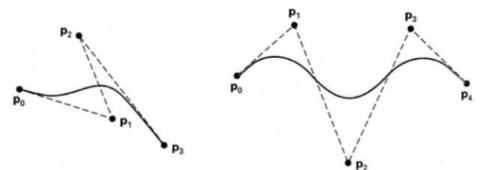
Variation-diminishing: curve lies in convex hull of points Cost: only interpolates endpoints
