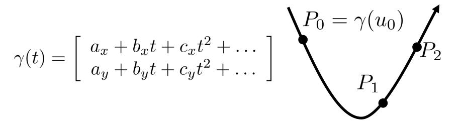
Notice: each coordinate is **linear combination** of a power of t
