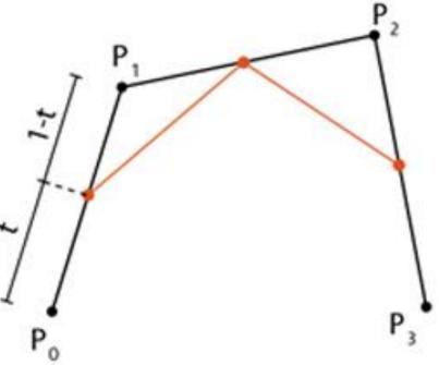
Main idea: recursive linear interpolation Start with four points – **control polygon** Clip corners
