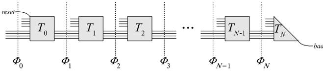
**Figure 2.** BMC unrolling of length  $N$ . The design is reset in the first frame and *Bad* is asserted in the last frame. The last frame is drawn partially because the next-state logic for the flops is not needed.
