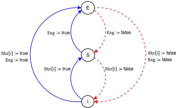
Fig. 1: State diagram of the German-ish protocol
