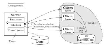
Figure 1. SMTSERVICE framework overview. The server implements Algorithm 1. Each client represents a different solver process in a computing node. Solid lines represent TCP/IP connections, while dashed lines represent disk I/O.
