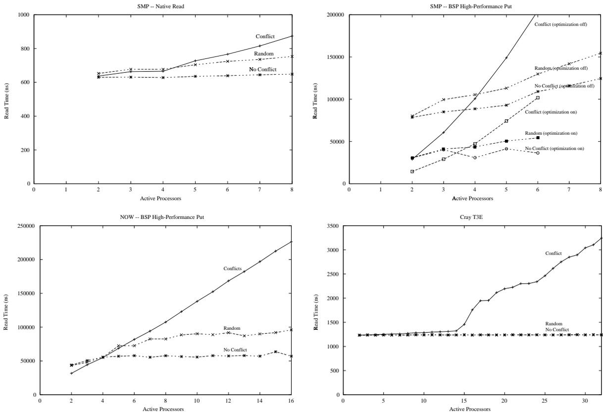
Figure 7: Remote memory access performance for the SMP, SMP-BSPlib, NOW-BSPlib, and Cray T3E architectures.
