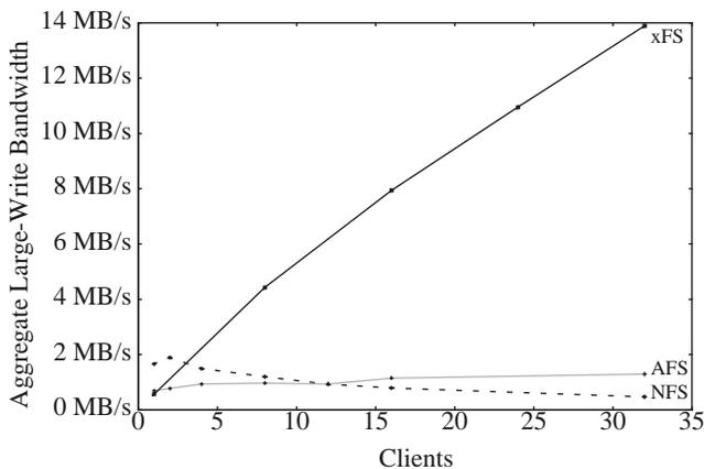
**Figure 8. Aggregate disk write bandwidth.** The x axis indicates the number of clients simultaneously writing private 10 MB files, and the y axis indicates the total throughput across all of the active clients. xFS uses four groups of eight storage servers and 32 managers. NFS's peak throughput is 1.9 MB/s with 2 clients, AFS's is 1.3 MB/s with 32 clients, and xFS's is 13.9 MB/s with 32 clients.
