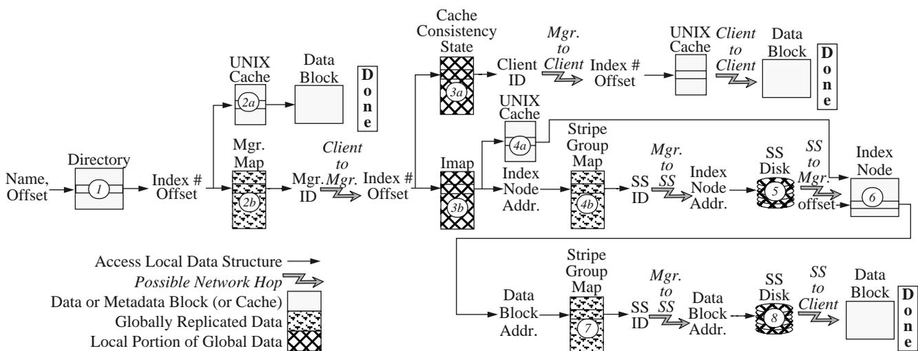
**Figure 3. Procedure to read a block.** The circled numbers refer to steps described in Section 3.2.1. The network hops are labelled as "possible" because clients, managers, and storage servers can run on the same machines. For example, xFS tries to co-locate the manager of a file on the same machine as the client most likely to use the file to avoid some of the network hops. "SS" is an abbreviation for "Storage Server."
