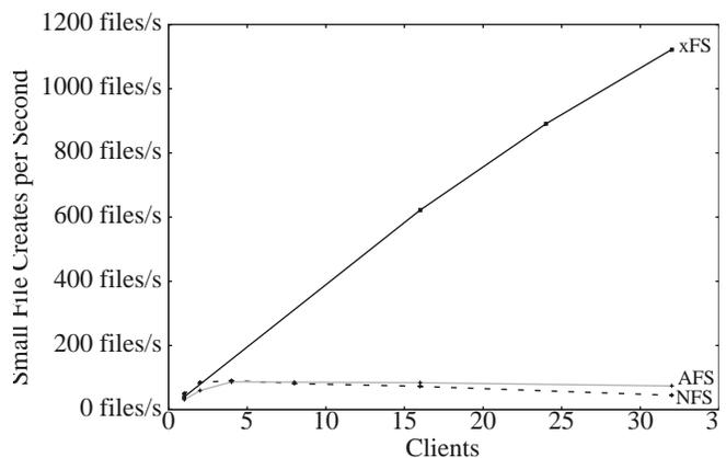
**Figure 10. Aggregate small write performance.** The x axis indicates the number of clients, each simultaneously creating 2,048 1 KB files. The y axis is the average aggregate number of file creates per second during the benchmark run. xFS uses four groups of eight storage servers and 32 managers. NFS achieves its peak throughput of 91 files per second with four clients, AFS peaks at 87 files per second with four clients, and xFS scales up to 1,122 files per second with 32 clients.
