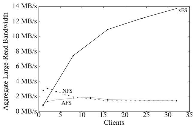
**Figure 9. Aggregate disk read bandwidth.** The x axis indicates the number of clients simultaneously reading private 10 MB files and the y axis indicates the total throughput across all active clients. xFS uses four groups of eight storage servers and 32 managers. NFS's peak throughput is 3.1 MB/s with two clients, AFS's is 1.9 MB/s with 12 clients, and xFS's is 13.8 MB/s with 32 clients.
