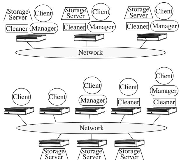
**Figure 2. Two simple xFS installations.** In the first, each machine acts as a client, storage server, cleaner, and manager, while in the second each node only performs some of those roles. The freedom to configure the system is not complete; managers and cleaners access storage using the client interface, so all machines acting as managers or cleaners must also be clients.
