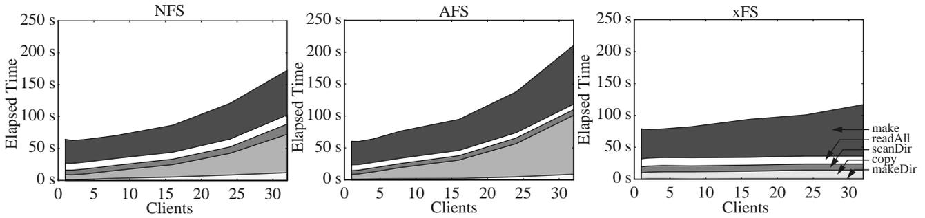
**Figure 11. Average time to complete the Andrew benchmark for NFS, AFS, and xFS as the number of clients simultaneously executing the benchmark varies.** The total height of the shaded areas represents the total time to complete the benchmark; each shaded area represents the time for one of the five phases of the benchmark: makeDir, copy, scanDir, readAll, and make. For all of the systems, the caches were flushed before running the benchmark.
