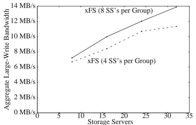
**Figure 12. Large write throughput as a function of the number of storage servers in the system.** The x axis indicates the total number of storage servers in the system and the y axis indicates the aggregate bandwidth when 32 clients each write a 10 MB file to disk. The 8 SS’s line indicates performance for stripe groups of eight storage servers (the default), and the 4 SS’s shows performance for groups of four storage servers.
