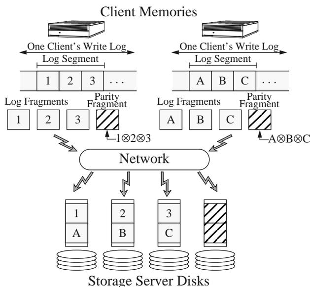
**Figure 1. Log-based striping used by Zebra and xFS.** Each client writes its new file data into a single append-only log and stripes this log across the storage servers. Clients compute parity for segments, not for individual files.
