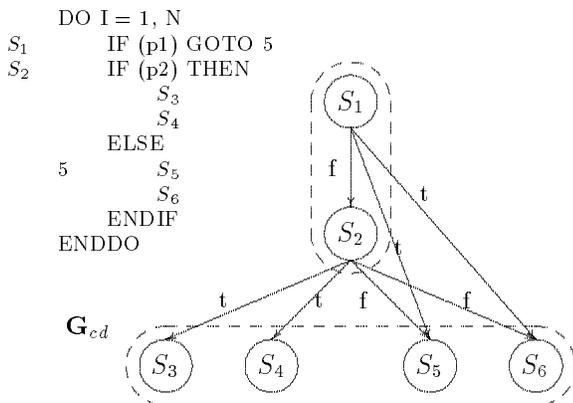
Distribution restructuring, label renaming, and code generation performed on the above results in the following code.
