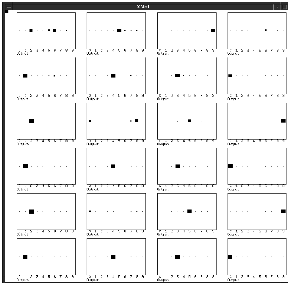
Figure 1: User identification with the NNID Network. The output layer of NNID is shown for each of the 24 test vectors in one of the 4 splits tested. The output units are lined up from left to right, and their activations are represented by the size of the squares. In this split there were two false alarms: one is displayed in the top right with activation 0.01, and one in the second row from the bottom, second column from the left with 0.35. All the other test vectors are identified correctly with activation higher than 0.5.
