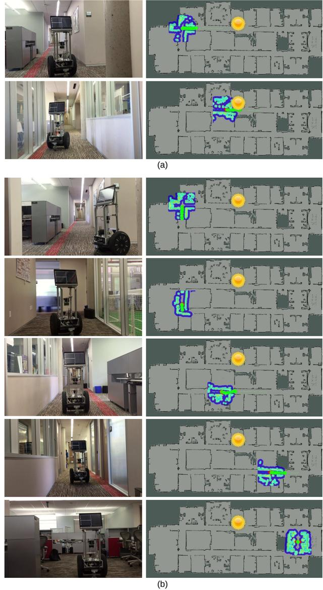
**Figure 2:** Screen shots of two illustrative trials: (a) Using the baseline approach (CORPP), the robot chose Route 1 that is dangerous but shorter, causing the robot to become unrecoverably lost in the “sunny” area; (b) By reasoning about current time (morning) and weather (sunny), iCORPP successfully helps the robot take Route 2 to avoid being trapped in the “sunlight” area, even though the route is longer.
