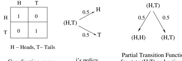
**Figure 1: Example of the partial transition function for state  $(H,T)$  in the Coordination game**
