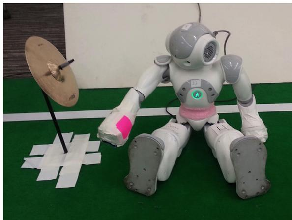
**Fig. 9.** The experimental setup with an Aldebaran Nao robot. The robot is placed in a sitting position, with a cymbal within arm's reach, and a square of pink taped to its hand. The learning agent can move either of the robot's right shoulder joints and can potentially hit the cymbal, push the button on its right foot, or move more or less pink into the view of its camera.
