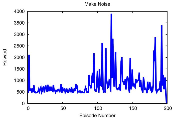
**Fig. 14.** Rewards received by the one successful trial of *TEXPLORE-VANIR* on the task of maximizing the energy received by the robot's microphone. Rewards greater than 800 represent times that the robot hit the cymbal with its arm.
