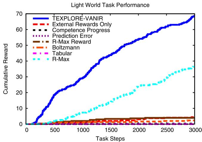
**Fig. 7.** Cumulative rewards received by each algorithm, using intrinsic and external rewards combined, over the 3000 steps of the task, averaged over 30 trials. TEXPLORE-VANIR receives the most reward, while the agent using only external rewards performs very poorly.
