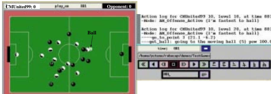
Fig. 1: The layered disclosure tool. The terminal window (top right) shows layered information for the instant shown in the graphical game display (left). On the control bar (bottom right), the “P” buttons control which player is being examined and the “L” buttons control the level of displayed information.
