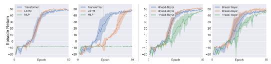
Figure 5: A study on neural architectures. We use a Transformer with 8-head attention and one Transformer encoder layer in MACTA experiments. **Left two:** Train attacker-only tasks using different neural architectures on two machines. **Right two:** Train attackers with different Transformer configurations on two machines.
