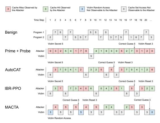
Figure 8: Example trajectories of different attackers and benign agents in a 8-set 1-way L1 cache. The number indicates the cache set being accessed. Red and green boxes show the observation by the attacker. The latency of other programs (i.e., victim or benign) cannot be observed by the attacker, but they can be observed by the detectors. The program IDs are randomized during training, and the attacker can be any of the two programs in the system. The cache is initialized with random states.
