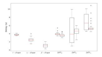
Fig. 4: Box and whisker plot of real-world experiments with various conditions. Details for each condition can be found in Table II. When the two robots use different conditions, the delay of each robot is plotted separately. Note that PHHP did not incur a single collision or turnaround behavior across all 192 experiments with various conditions.
