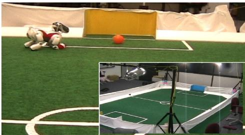
Fig. 1. An Image of the Aibo and the field. The robot has a limited field-of-view of  $56.9^\circ$  (hor) and  $45.2^\circ$  (ver).
