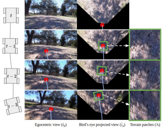
Fig. 1: Overview of the Visual Patch Extraction process at time  $t$ . The robot’s next location  $\tilde{x}_t$  is estimated (red circle) based on current velocity, and a visible image patch of terrain at the same consistent location  $\tilde{x}_t$  is extracted from bird’s eye view images from previous timesteps of different viewpoints.
