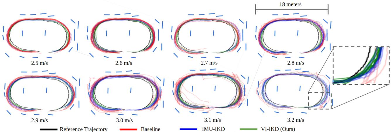
Fig. 5: Trajectory traces for the indoor experiments where the vehicle tracks a reference trajectory counter-clockwise at different speeds. The inset shows Turn 1 as executed by the vehicle at  $3.2\text{m/s}$  using the three approaches. We see that VI-IKD is able to track the reference trajectory more accurately than IMU-IKD [6], confirming our hypothesis. Blue lines along the track show the virtual fixtures used as a map for vehicle state-estimation using EnML [34].
