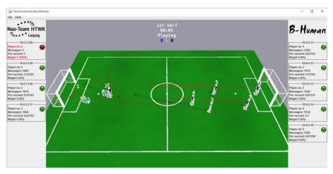
**Fig. 2** Team Communication Monitor during a normal Standard Platform League game. The centered 3-D view displays the current world states, i.e. position, status, and ball position, communicated by the playing robots. The side views show the status and the frequency of each robot's communication
