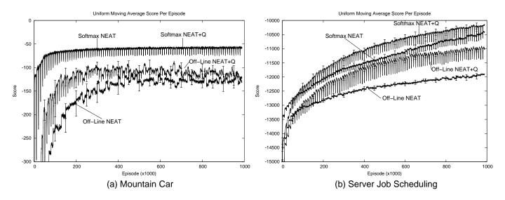
Figure 7: The performance of combining evolutionary function approximation with on-line evolutionary computation compared to using each individually in the mountain car and server job scheduling domains.
