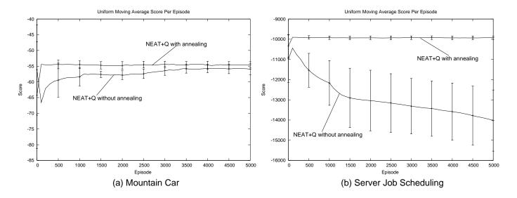
Figure 11: A comparison of the performance of the best networks evolved by NEAT+Q when tested, with and without annealing, for an additional 5,000 episodes.
